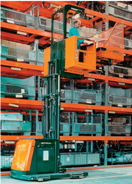
Various types of fork-lift truck with integrated draw-wire sensor.
