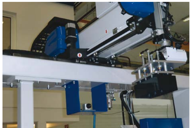
moldCONTROL thermal imaging camera on the traverse of a handling system
