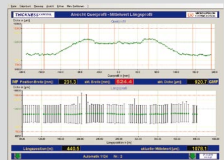
Combination profile TIP 8301.EO; vertical cursors show the points which are used for calender control
