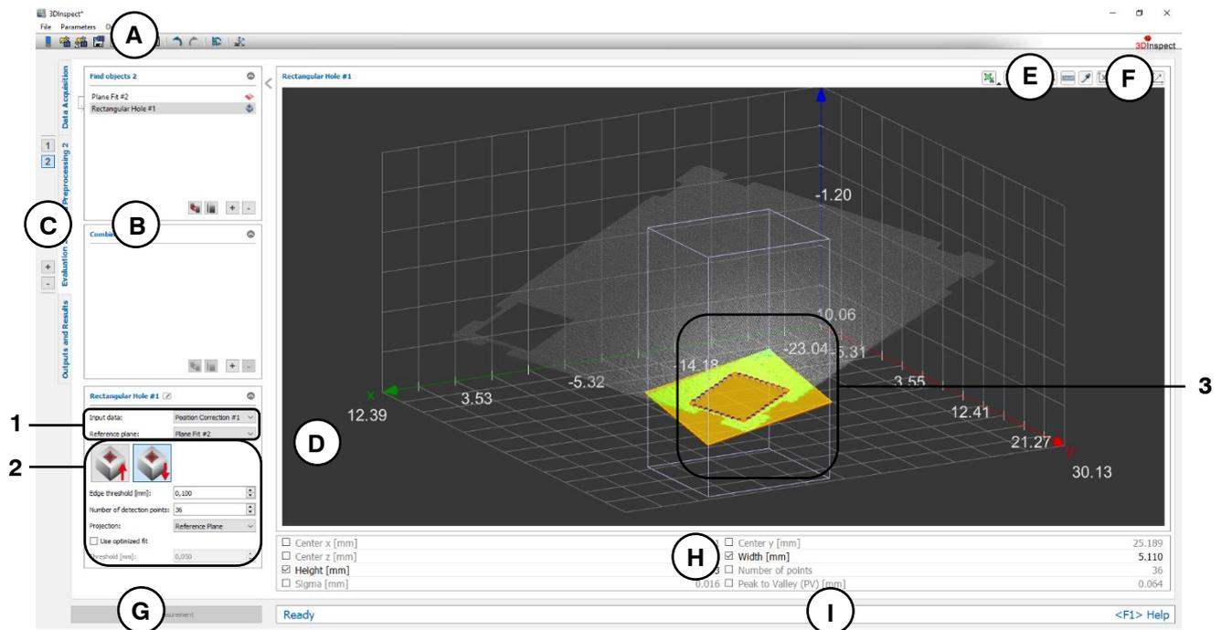
Fig. 6.11: "Rectangular Hole" Measuring Program
