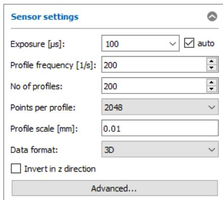
Fig. 3.12: "Sensor settings" box (scanCONTROL 30XX)
