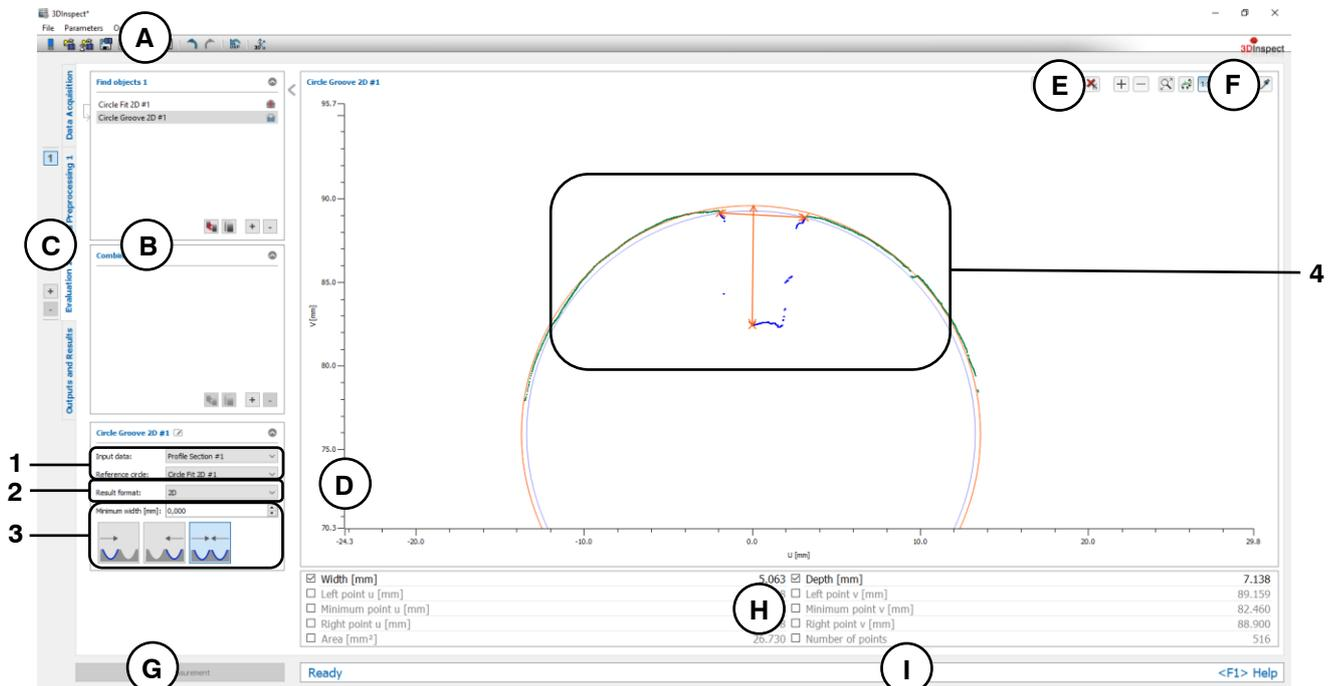
Fig. 6.27: "Circle Groove 2D" Measuring Program
