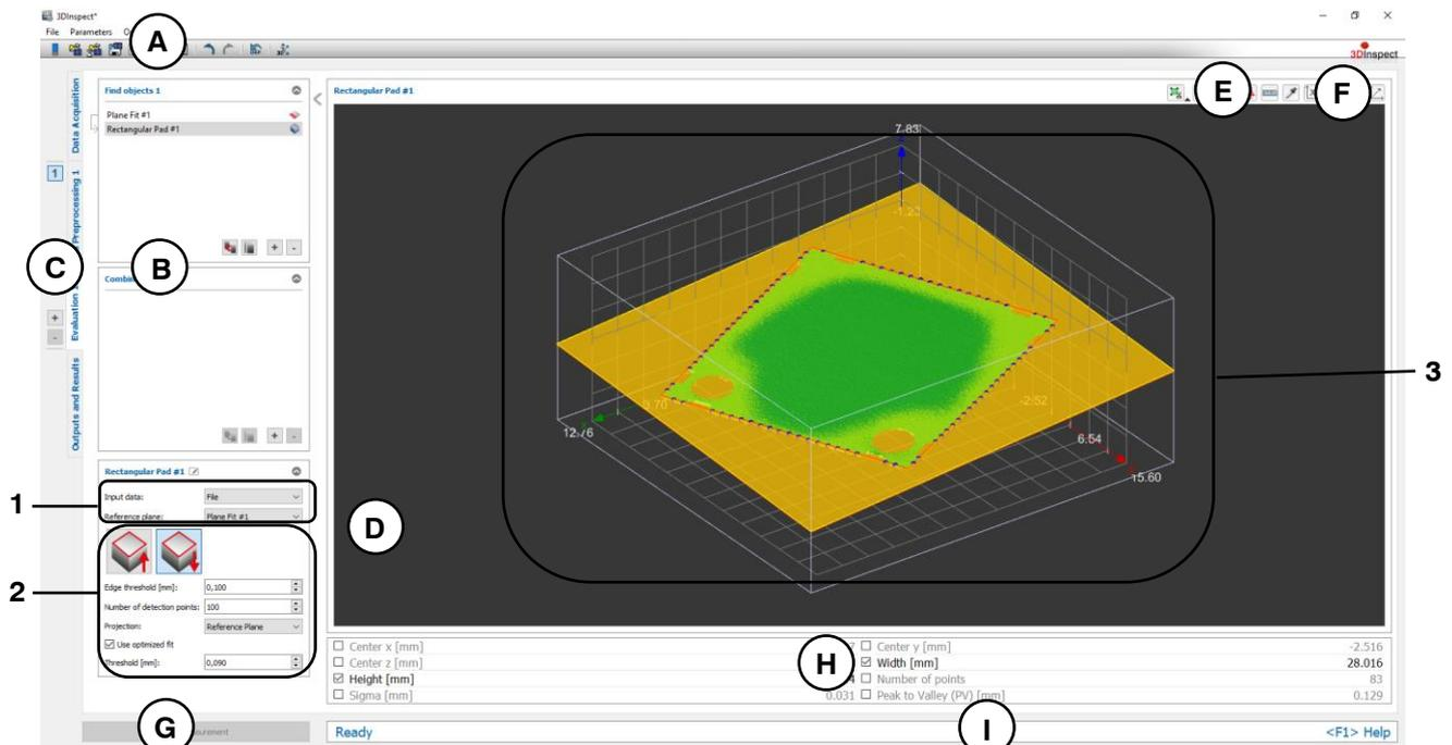
Fig. 6.12: "Rectangular Pad" Measuring Program
