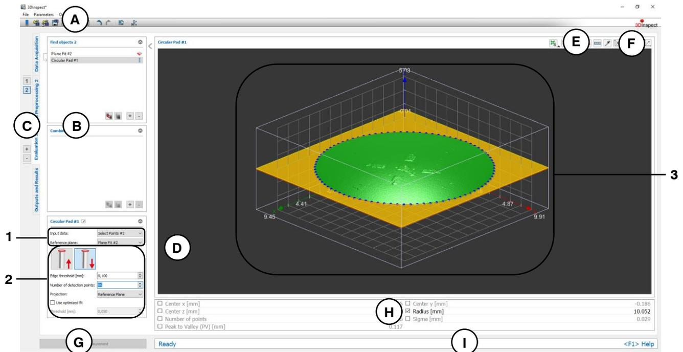
Fig. 6.10: "Circular Pad" Measuring Program
