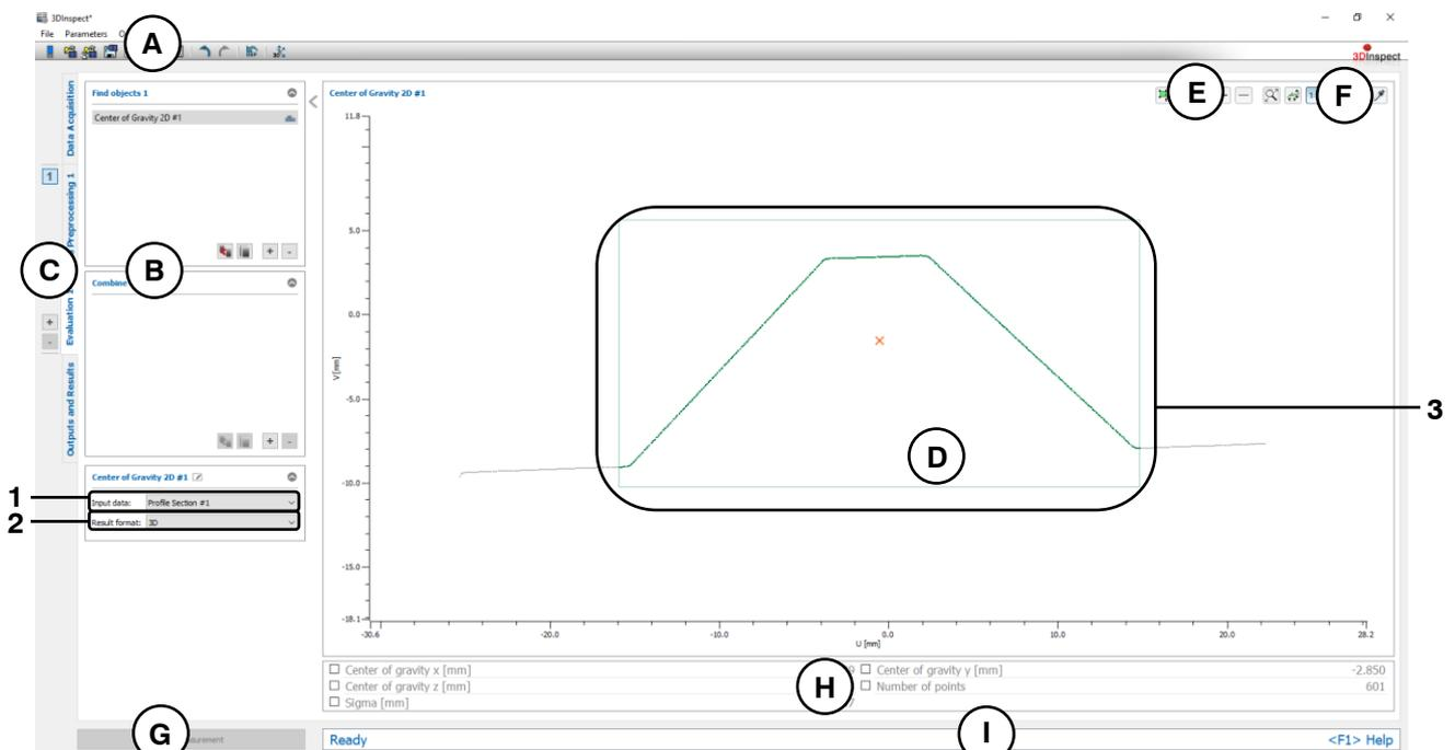
Fig. 6.17: "Center of Gravity 2D" Measuring Program
