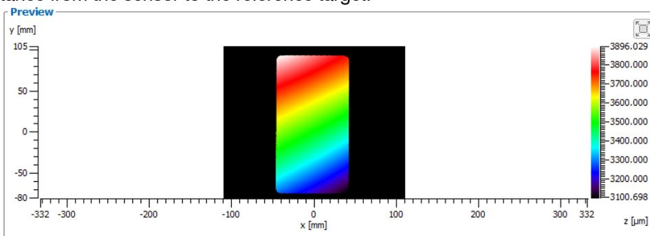
Fig. 3.8: Positioning the reference object – Distance too small
