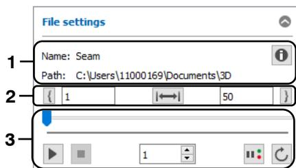
Fig. 3.18: Settings in offline mode – single file ("2D" data format)
