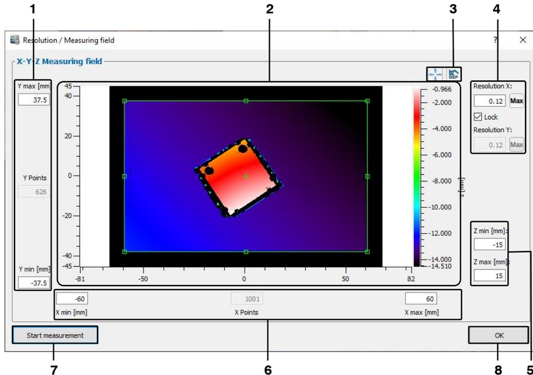
Fig. 3.14: "Resolution / Measuring field" dialog box
