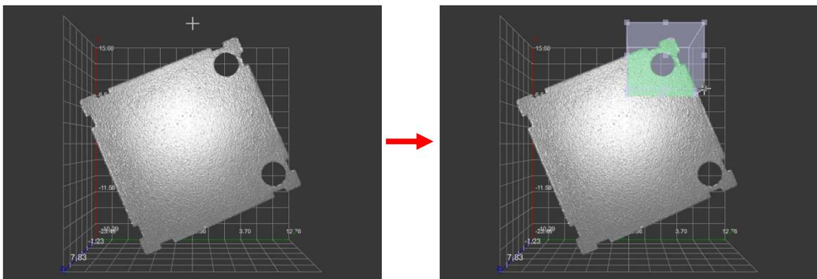
Fig. 3.63: Setting the complete ROI (x/y range)
