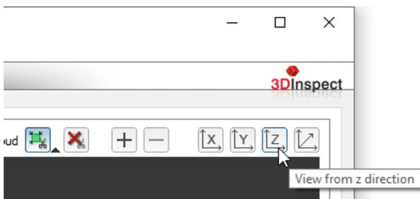
Fig. 3.62: Viewing the point cloud from the z direction
