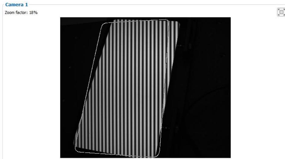
Fig. 3.6: Positioning the reference target – position has to be corrected
