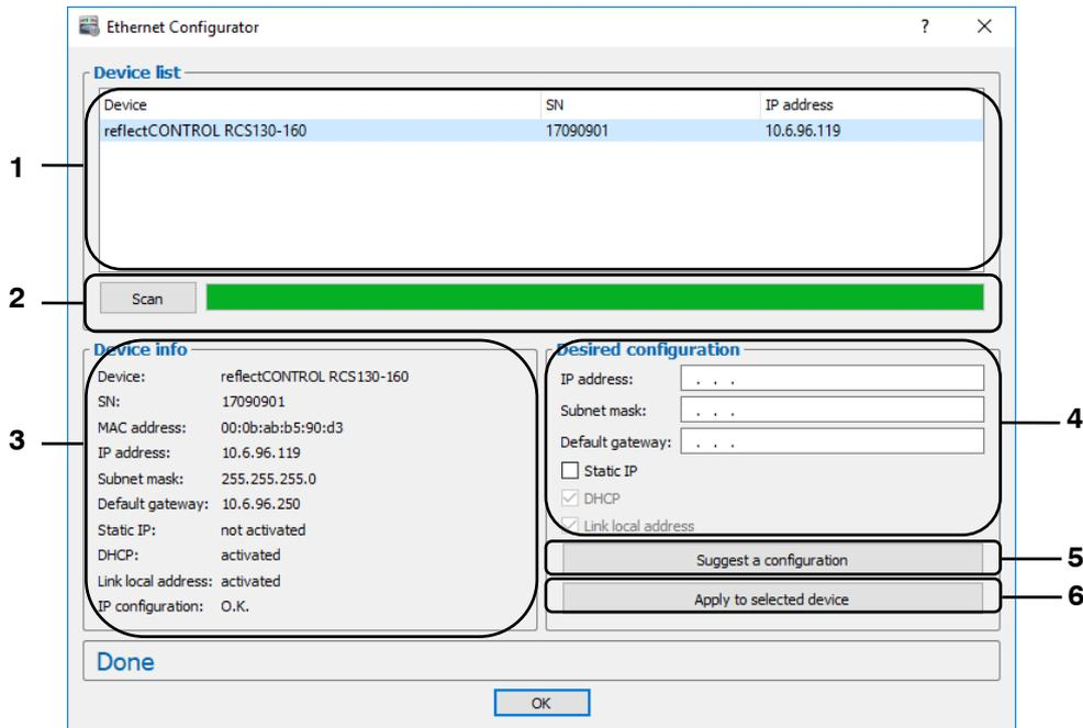
Fig. 3.90: "Ethernet Configurator" dialog box
