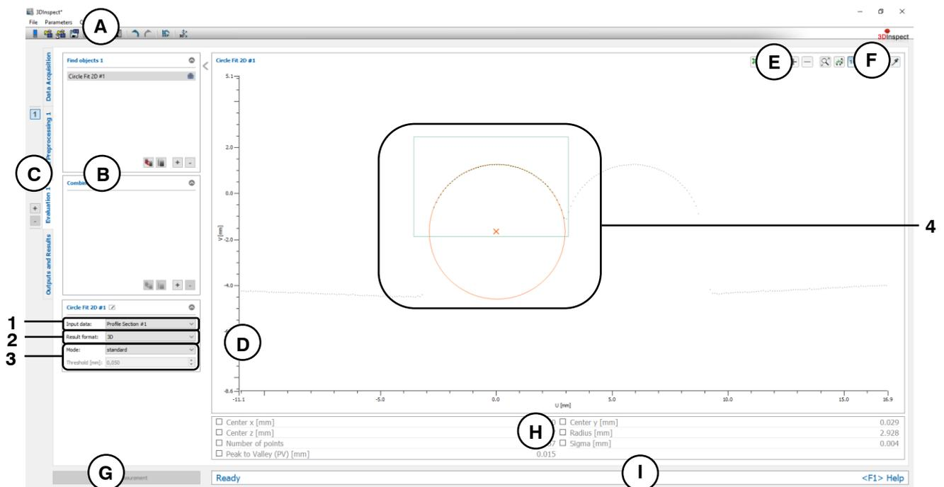
Fig. 6.20: "Circle Fit 2D" Measuring Program
