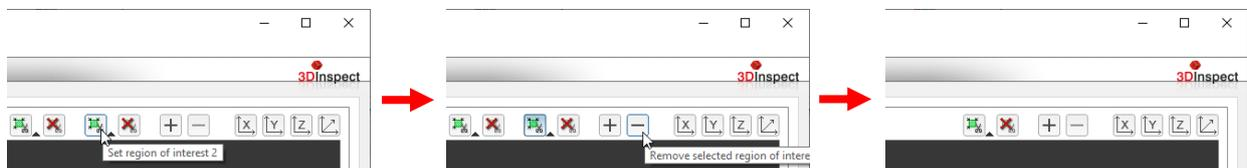
Fig. 3.74: Removing a ROI
