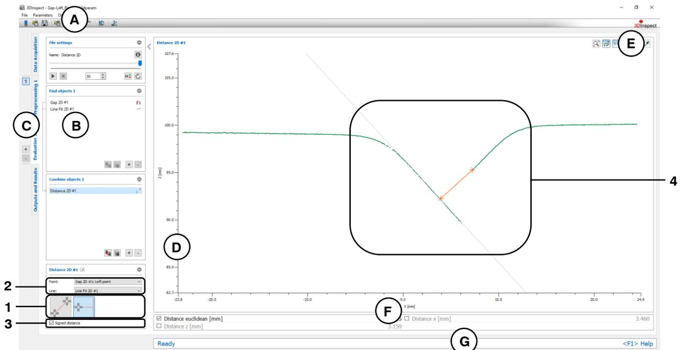
Fig. 6.37: "Distance 2D" Measuring Program
