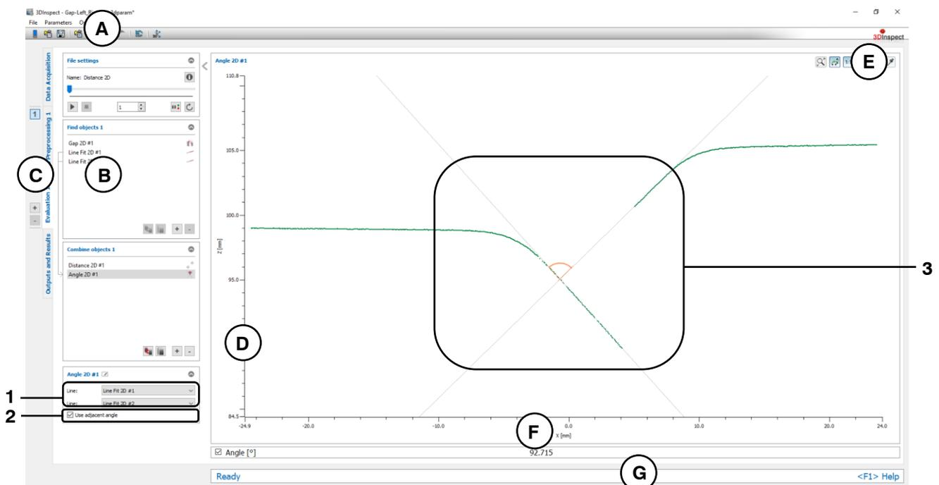
Fig. 6.38: "Angle 2D" Measuring Program
