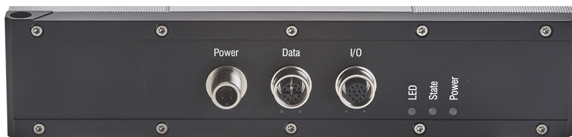
Fig. 13 Arrangement of connections
