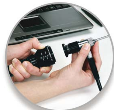
Attachment of camera and lens onto endoscope
