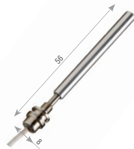
EDS-28-G-CA-U Rugged inductive miniature sensor with in the cable integrated electronics ▪ Miniature actor for formula 1 ▪ Measuring range 28mm ▪ Pressure resistance up to 350bar
