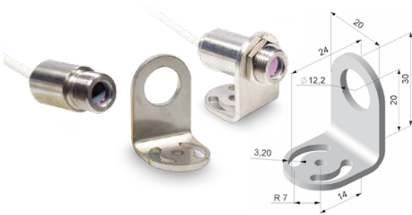
TM-FB-CT Mounting bracket, adjustable in one axis
