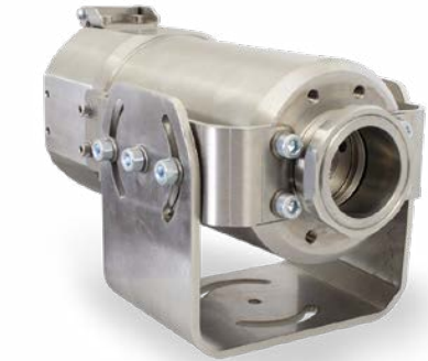
TM-J-CTL Cooling jacket (length 228mm, ø 89mm) with adjustable mounting bracket TM-JAB-CTL; suitable for ambient temperatures up to 180°C
