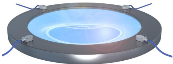
Right: 4 capacitive sensors measure the tilt of the lens carrier
